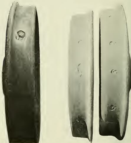
Fig. 4—Shelled Out Wheels.
